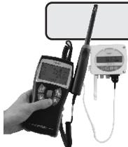
The EHK 500 is a reference portable instrument (optional) which enables you to adjust at one point the humidity and temperature reading, via the RS 232 connection cable. Thanks to this new time-saving system, no need to return the transmitter to our factory.
